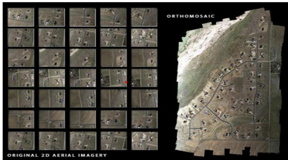
Figure 7. An example ortho mosaic image is prepared using photogrammetry software (Source: https://medium.com/new-farmer/what-is-an-orthomosaic-photo-11140c0601pdf )
