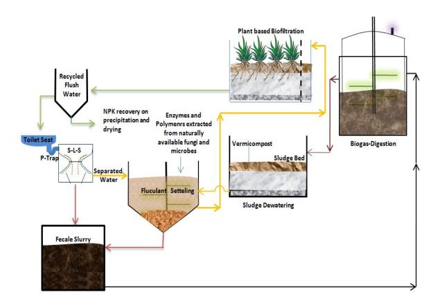
Figure 3.10: Schematic diagram of Zero Discharge Toilet System
