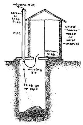
Figure 3.2: Schematic diagram of a Ventilated Improved Pit Latrine Source: http://www.ugandanetwork.org.uk
