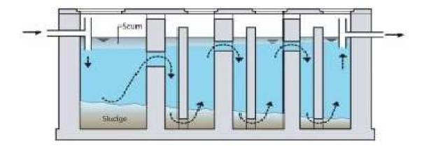
Figure 4.2: Schematic cross-section of an Up-Flow Anaerobic Baffled Reactor Source: Morel and Diener, 2006 [27]
