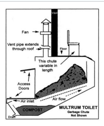
Figure 3.3 General schematic diagram of a Composting Toilet Source: Adapted from the Humanure Handbook
