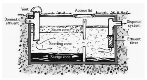
Figure 4.1: Schematic of a Septic Tank, Source: http://www.nrc.govt.nz
