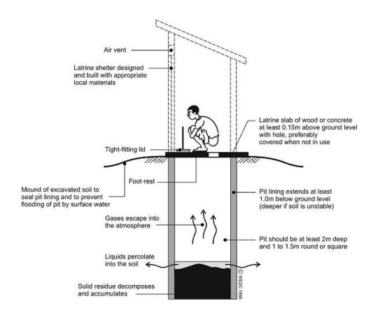
Figure 3.1: Schematic diagram of a simple pit latrine. Source: Harvey et al. 2002 [12]
