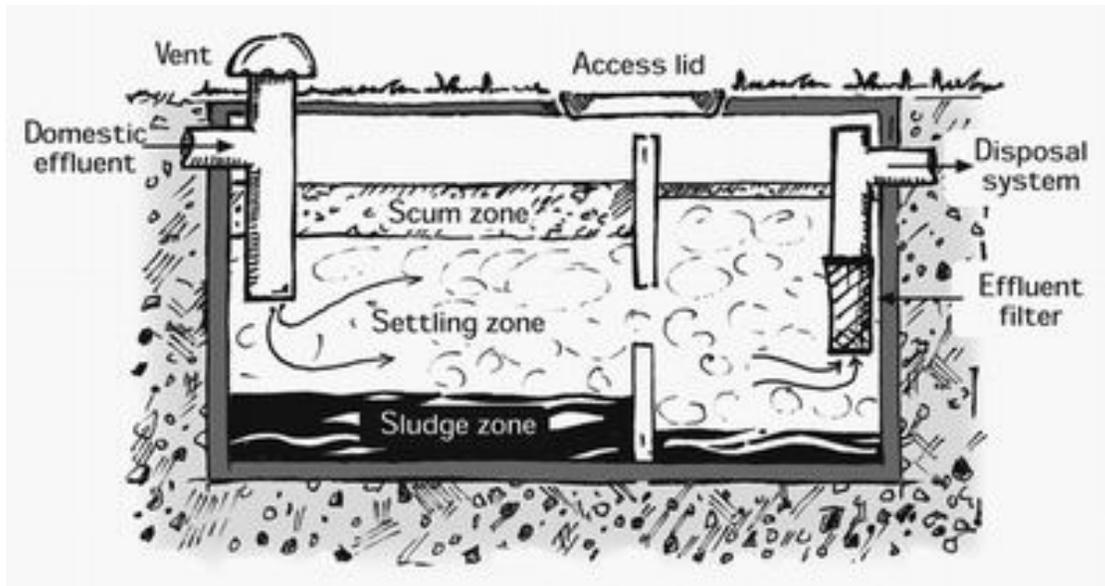
**Figure 4.1: Schematic of a Septic Tank, Source: <http://www.nrc.govt.nz>**
