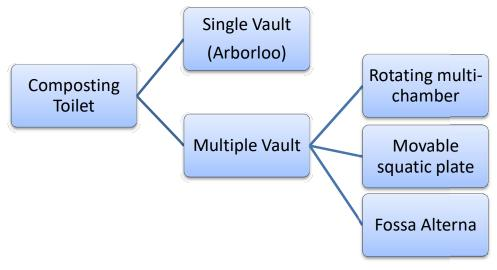
Figure 3.4 Classification of Composting Toilets, according to GTZ, 2010 [15]
