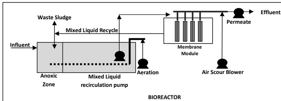
**Schematic Diagram of a Membrane Bioreactor**
