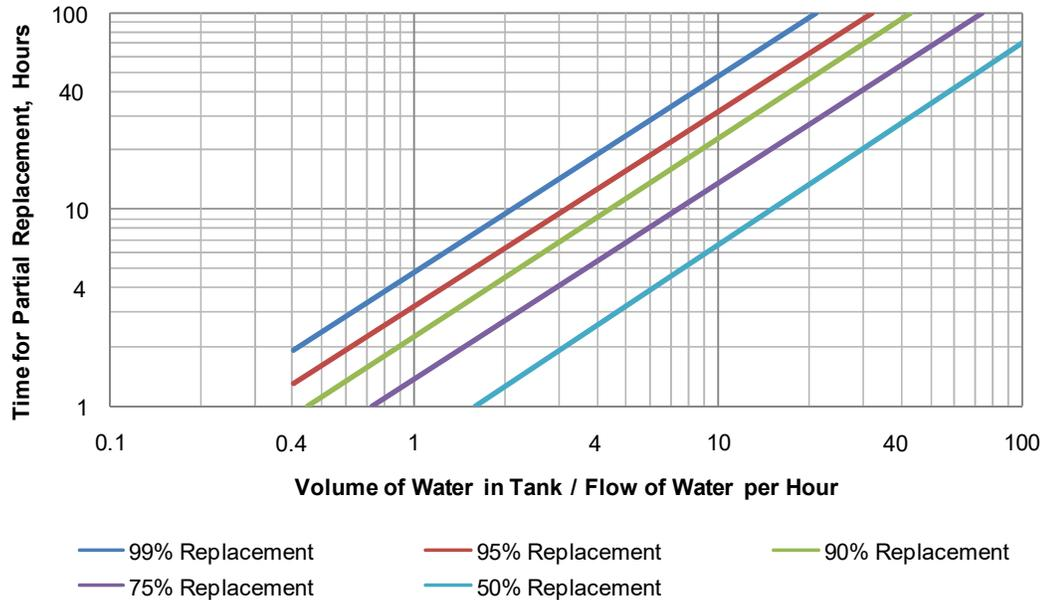
**Figure 3: Approximate times required to replace water in test chambers in flow-through tests (For Example: For a chamber containing 4 L, with a flow of 2 L/h, the above graph indicates that 90% of the water would be replaced every 4.8 h. The same time period, such as hours, must be used on both axes, and the same unit of volume, such as liters, must be used for both volume and flow (Adapted from USEPA, 2002)**
