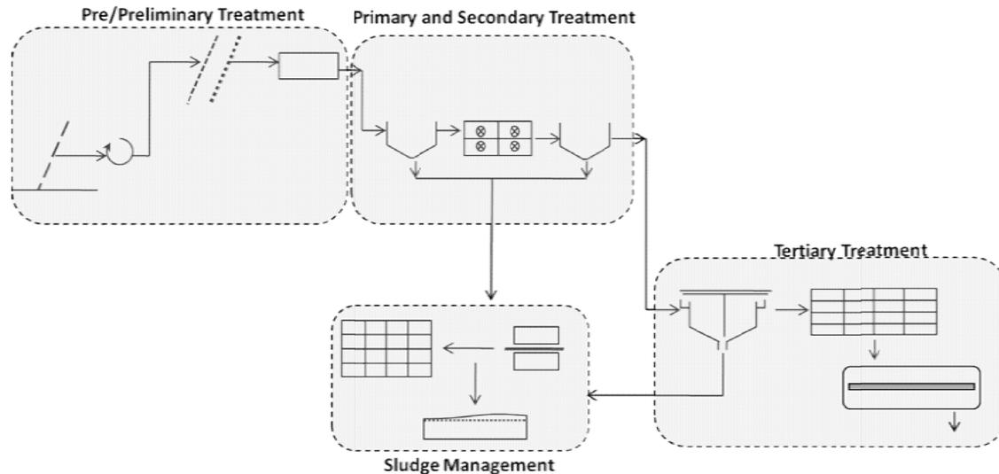
**Figure 1: Process Chain for Sewage Treatment**
